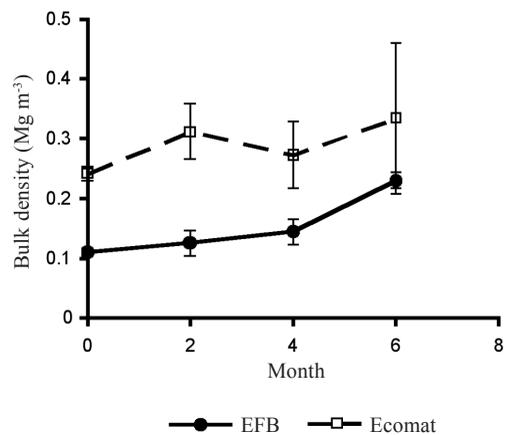
*Fig. 2: Bulk density of EFB and Ecomat*
