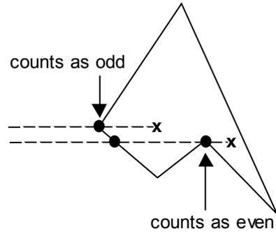
Figure 2. (a) The inside test method, and (b) the intersection with a polygon vertex
