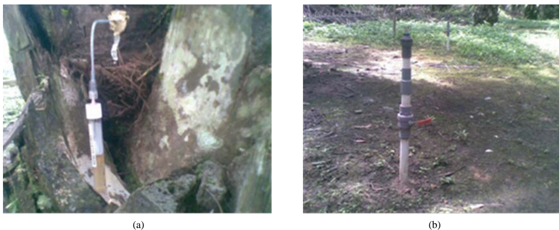
Figure 1. (a) A micro sampler; (b) PVC vacuum pipe.
